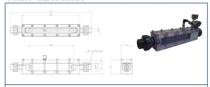
Distribution GasVolume: <u>1.25L/min(max)</u> 0.2Mpa=29psi g
