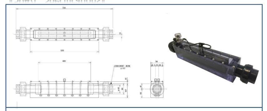
Distribution GasVolume: <u>10L/min(max)</u> 0.2Mpa=29psi g
