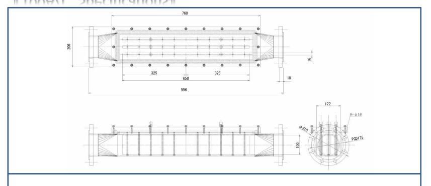
Distribution GasVolume: 30L/min(max) 0.2Mpa=29psi g
